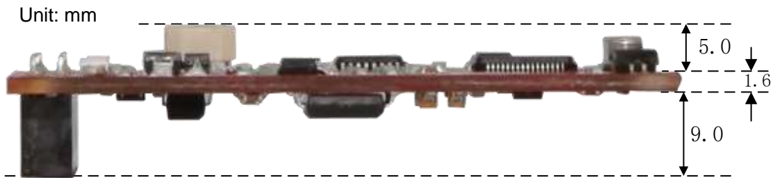
Figure 1.5 Front Back Height Dimensions of HART Module
